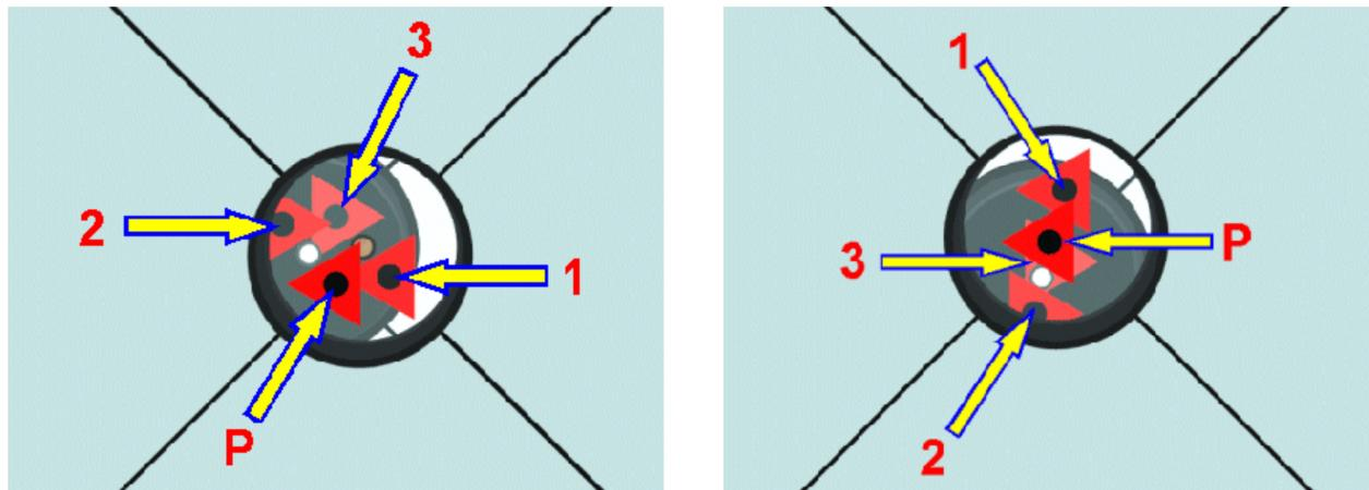
▲ Reflection "P" is the "Primary" or "first" reflection and is the direct reflected image of the spot itself via the Diagonal mirror after 1 FL pass. Reflection "P" is what is visible "without" the autocollimator whereas images (#1, #2, & #3) are reflections of "P"
